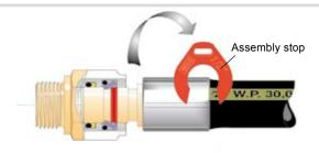
Using a screwdriver, remove the assembly stop.
